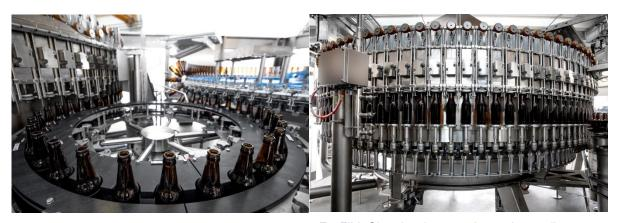
The re-designed handling parts, which are now lighter and smaller, ensure a changeover time shorter than 30 minutes with one operator.
