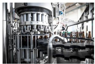
The ultra-clean crowner manufactured by Sidel, with its open design and off-set crowning ring, adds further performance to the bottling process with no internal lubrication needed.
